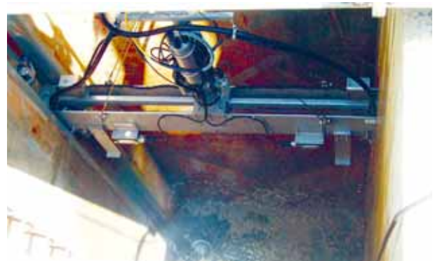
図7 清掃機降下状況 Fig. 7 Operating conditions of the cleaning system of square ditch
