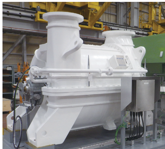
図11 Reaction furnace blower工場試験 Fig.11 FAT for reaction furnace blower
