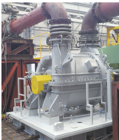
図10 Combustion air blower工場試験 Fig.10 FAT for combustion air blower
