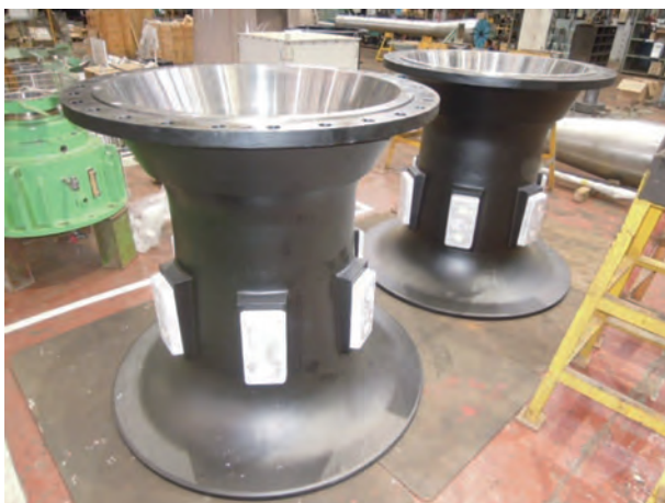
図3 循環水ポンプ 吸込ベルとアルミ陽極 Fig.3 View of the Circulating water pump suction bell and sacrificial anode
