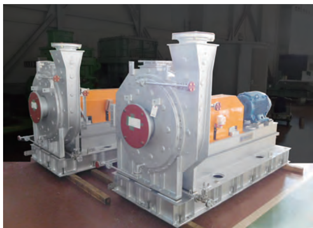
図3 Sulfur fume Blower外観 Fig.3 View of Sulfur fume blowers
